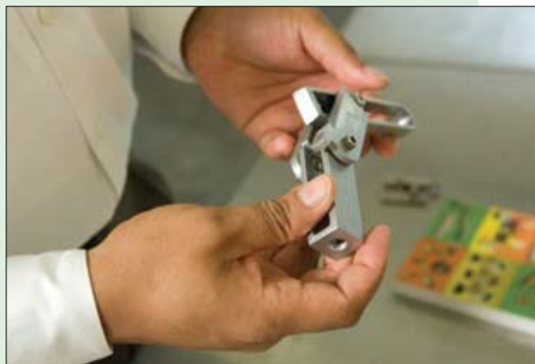
Fields examines a prototype hinge for his new window design.
